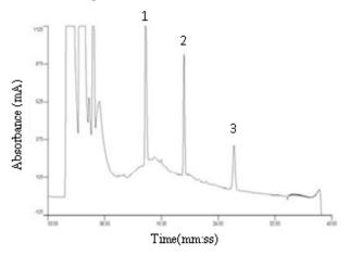
**Fig 1.** HPLC chromatograms of the mixture of standard biogenic polyamines ( $10 \mu g \text{ ml}^{-1}$ ) derivatized according to Method 3, gradient elution 3 and wavelength 254 nm. . Peaks identification: 1) putrescine; 2) spermidine and 3) spermine (14-27 min).
