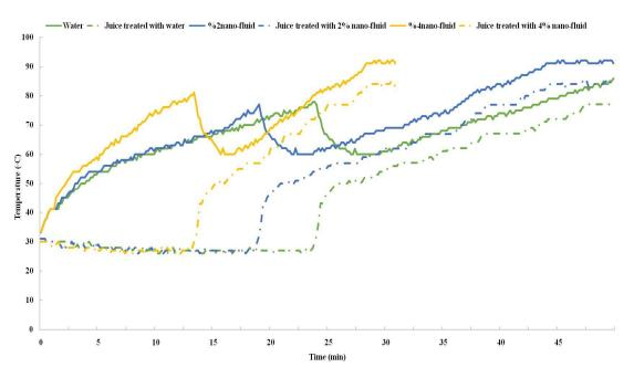
**Figure 2:** Temperature changes and time reduction during the thermal processing of watermelon juice by 2% and 4% alumina nano-fluid compared with water
