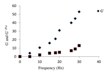
Figure 5. Variation diagram of the elastic (G') and viscose (G") coefficients for the optimal samples of walnut husk pectin at 1% concentrations
