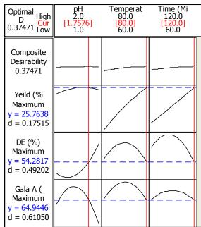
**Figure 4.** Optimization diagram of the pectin extraction conditions based on the efficiency rate, esterification degree and galacturonic percentage of the pectin samples extracted from walnut green husks
