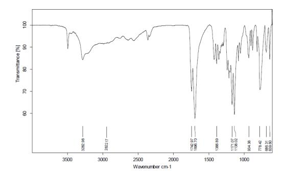
Figure 6. FTIR absorption spectrum of the optimal pectin sample isolated from walnut green husk
