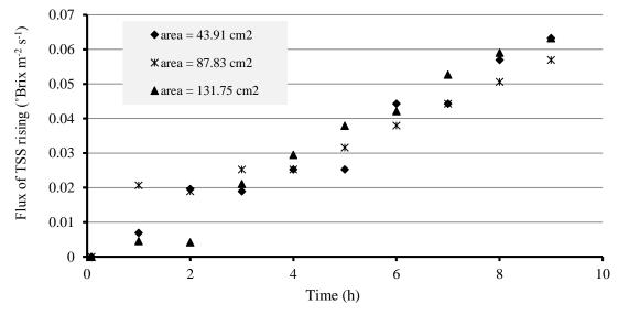
Fig. 9. Flux of the total soluble solid (TSS) rising during membrane concentration of the red beet juice
