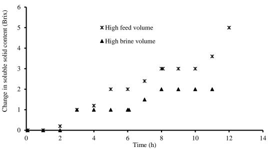
Fig. 5. Effects of feed and brine volumes on changes in soluble solid content of feed during membrane concentration of the red beet juice
