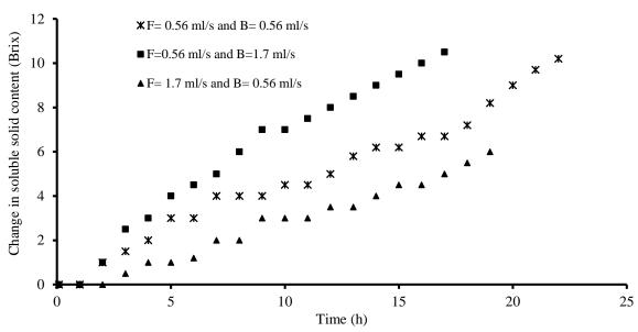
**Fig. 7**. Effects of the fluid velocity on the soluble solid content of feed during membrane concentration of the red beet extract (F, feed flow rate; and B, brine flow rate)
