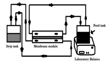
Fig. 1. Scheme of the osmotic distillation unit
