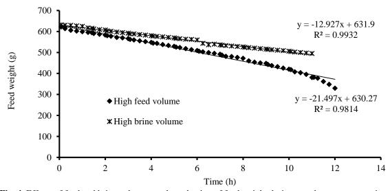
Fig. 4. Effects of feed and brine volumes on the reduction of feed weight during membrane concentration of the red beet juice
