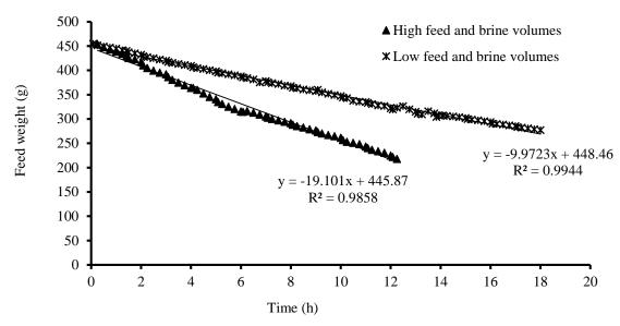
Fig. 2. Effects of feed and brine volumes on the feed weight during membrane concentration of the red beet juice
