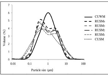
Figure 2. Particle size distribution of milk samples
