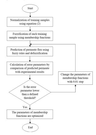
**Figure 2.** Proposed algorithm for parameters modification of membership functions
