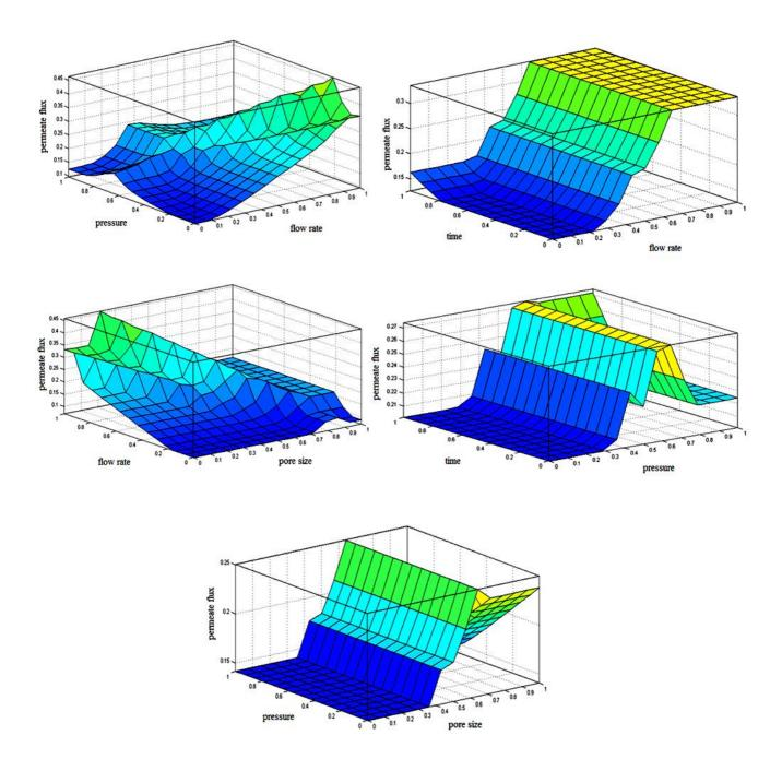
**Figure 3.** The relationship between model input and output parameters considering the modified membership functions and fuzzy rules
