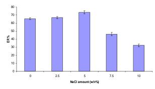
Fig. 2. Effect of NaCl amount on the extraction efficiency of DEHP
