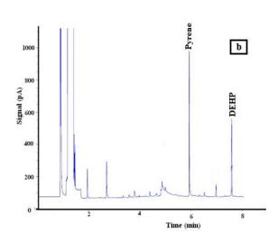
Fig. 4. GC-FID chromatograms of boiled water already cooled down inside a polyethylene glass, before (a) and after (b) spiking with  $1.0 \mu g L^{-1}$  of the plasticizer.
