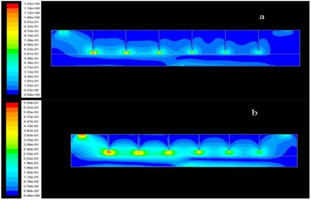
**Fig. 4.** Velocity contour in baffled module with channel height of 2 cm, baffle angle of 90° and 2 mm distance between baffles and membrane surface.
