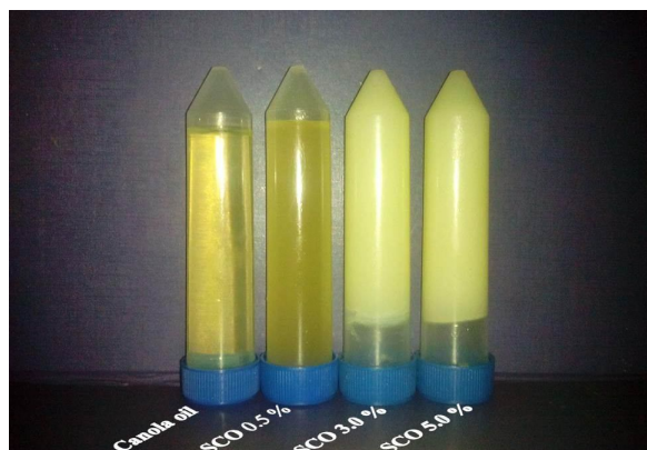
Fig. 2. The visual appearance of structured canola oil (SCO) samples crystallized at room temperature for 2 h. SCO: Structured canola oil
