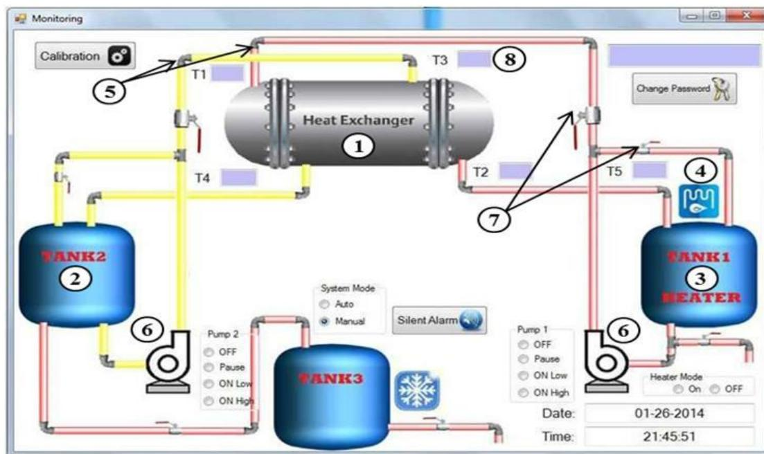
**Figure 1:** Simulation of intelligent nano-fluid heating system in the computer: insulated stainless steel shell and tube heat exchanger (1), food liquid reservoir (2), nano-fluid reservoir (3), heater (4), pipes of fluid flow (5), stainless steel centrifugal pump (6), stainless steel valves for fluid flow controlling (7), and pt 100 Sensors (8).
